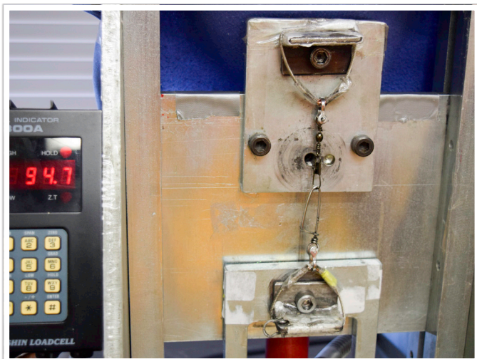
All swivels undergo batch load testing
