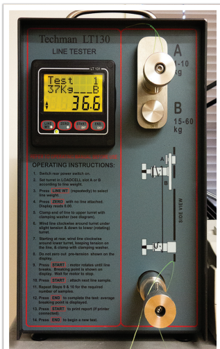
IFGA line is batch tested to ensure it breaks under it's nominated line class
